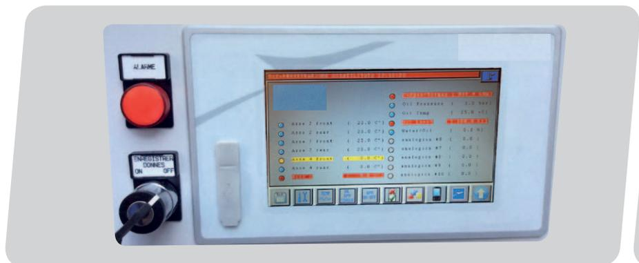
STRESSBOX MONITORS AND RECORDS ON A USB PEN-DRIVE AND IT TRANSMITS VIA SMS AND ETHERNET
