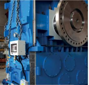
STRESS**BOX** MONITORS AND RECORDS ON A USB PEN-DRIVE AND IT TRANSMITS VIA SMS AND ETHERNET
